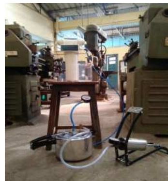
Efficient ultrafiltration unit for rural households utilizing available resources
